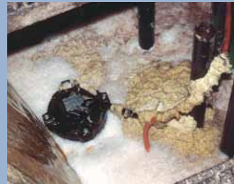
One of two S pumps used at a glass wool manufacturing plant for pumping process water with a high content of abrasive particles.
