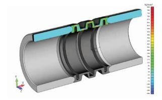
The geometry of the locking sleeve has been calculated with the help of the finite element method (FEM). The exercise was to guarantee the power transmission by the initial load between the rotating parts with different thermal characteristics of the materials (different expansion coefficient between SSiC and stainless steel 1:4), at temperatures up to 350°C (662°F).
